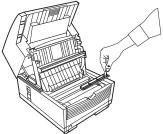
Install a new toner cartridge. See "Maintenance, Replacing the Toner Cartridge."
